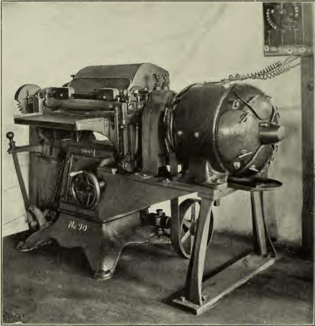
LIGHT SURFACING MACHINE, DIRECT-CONNECTED TO ELECTRIC MOTOR.
